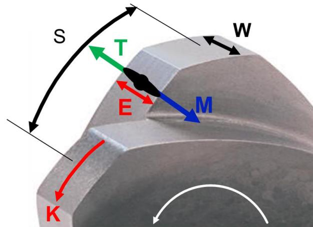
Figure 2: Kneading block key dimensions: stagger angle (W) and disc width (S). T indicates down-channel material transport, M represents back flow (distributive mixing) and E represents Extensional Flow (dispersive mixing) and K is the shear associated with any material that passes over the element crest.
