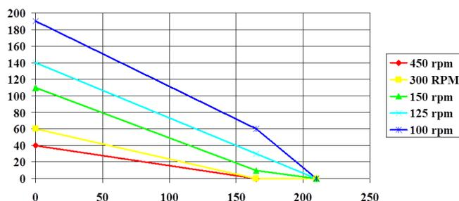
Figure 11:  $dP/dL$  as a function of rpm for narrow 3-lobe KB series with a 30/30 conveying element at the end.
