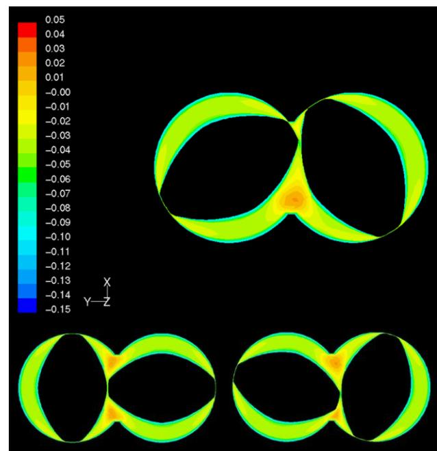
Figure 3: Simulation of axial velocity due to element rotation and material compression in the apex region.
