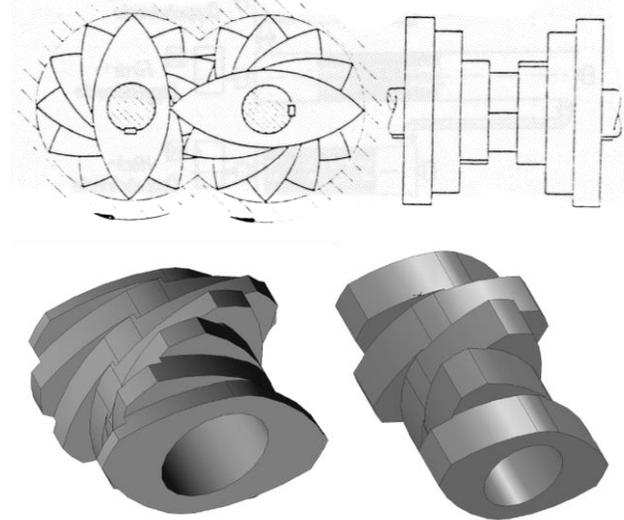
Figure 1: Comparison of original kneading block design (top) vs. the current standard kneading block (below).
