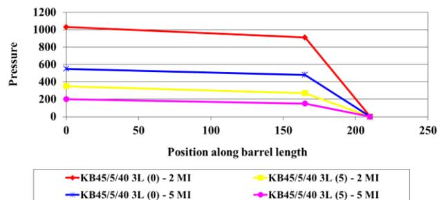
Figure 12: Impact of material Melt Index on pressure drop and  $dP/dL$
