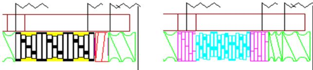
Figure 4: Examples of KB series with restrictive and conveying end elements.
