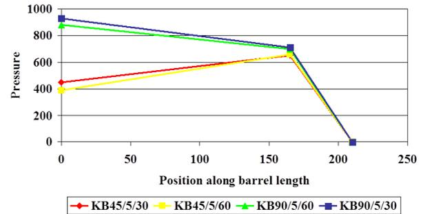
Figure 5: Effect of disc width and stagger angle on pressure build up and pressure drop characteristics.
