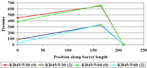
Figure 6: Impact of restrictive pressure on pressure build up efficiency of forwarding elements with respect to disc width.
