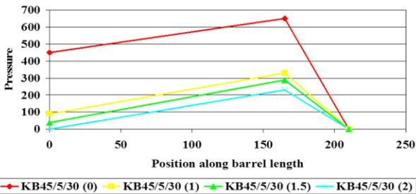
Figure 7: Impact of restrictive pressure value on pressure build up efficiency in 2 lobe kneading blocks.
