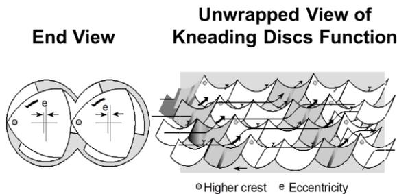
Figure 8: 3-lobe kneading block material flow.
