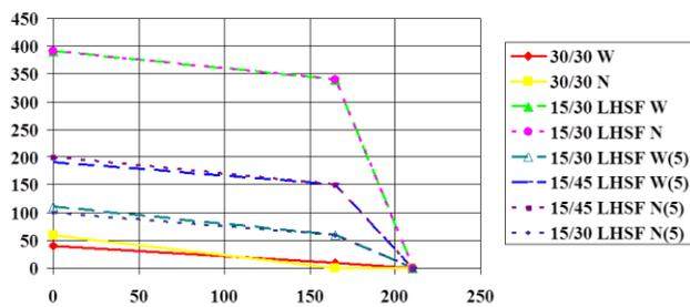
Figure 10: Pressure drop comparison across wide and narrow disc width 3-lobe kneading blocks.
