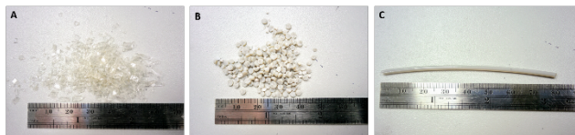
Figure 1. Optical images of recycled polyethylene terephthalate, (A) shredded, (B) pelletized, (C) filament.
